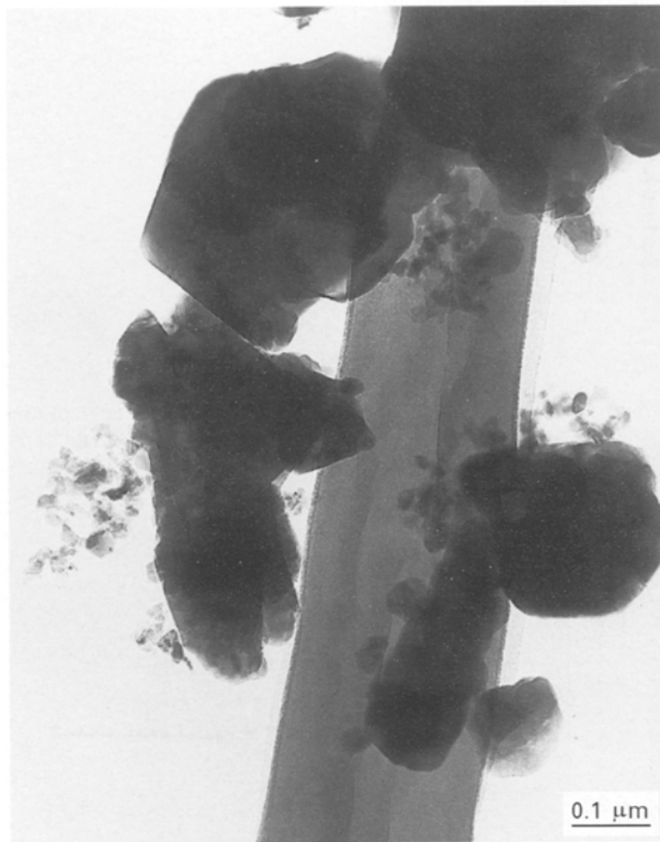
Figure 4 Transmission electron micrograph of \alpha - \text{Si}_3\text{N}_4 from “as-is” pyrolysed rice hulls.
